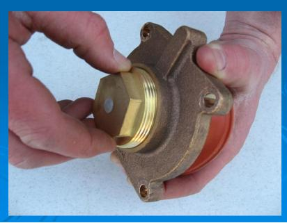
Form the large diaphragm so that the bead is properly seated in the bore of the RV cover.
