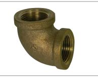
A.Y. MeDonald Mfg. Co. Pipe Fittings & Nipples are constructed from heavy duty brass and are rated for commercial, industrial and residential applications up to 125 WOG. Threads conform to ANSI B1.20.1 and fitting dimensions comply with ANSI B16.15.
