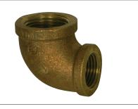
A.Y. M<sup>o</sup>Donald Mfg. Co. Pipe Fittings & Nipples are constructed from heavy duty brass and are rated for commercial, industrial and residential applications up to 125 WOG. Threads conform to ANSI B1.20.1 and fitting dimensions comply with ANSI B16.15.
